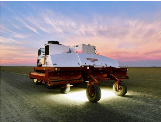
Carbon Robotics' Autonomous weeder uses AI-driven lasers instead of pesticides
